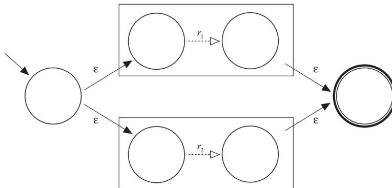
In this new machine there is a new start state with  $\epsilon$ -transitions to the two original start states and a new accepting state with  $\epsilon$ -transitions from the two original accepting states (which are no longer accepting states in the new machine). Clearly the new machine has a path from the
